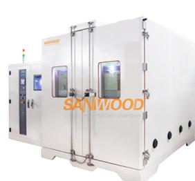
Walk in Battery Explosion Proof High & Low Temperature Chamber
